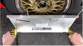
The rear tape measurement (side towards the rear of the vehicle) minus the front tape measurement (side closest to the front of the vehicle) is the total toe of the axle. A larger measurement on the front side indicates toe out, and a larger measurement on the rear side indicates toe in. For example, if the front measurement is 66° and the rear measurement is 66 3/32 the axle has a total toe in of 3/32°.
