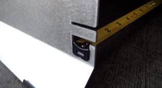
**Step 4: Measure Toe**Check that the stand-offs on both plates are properly seated against the rim of the wheels.
