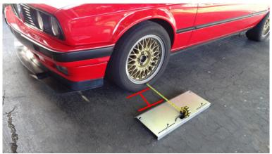
Center the steering wheel. Lay the plain toe plate (plate without the integrated camber gauge) down on the ground approximately 8" from the tire. The bottom of the plate should be pointing toward the vehicle.
