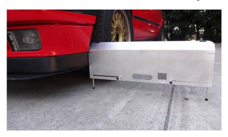
**<u>Tip:</u>** If it is desired to simply add a certain amount of camber, the gauge can also be calibrated on the wheel itself. For example if you are out at the track and decide you want to add 1 degree more negative camber, the gauge can be placed on the wheel and zeroed. Now camber can be adjusted until the gauge reads 1 degrees negative camber.
